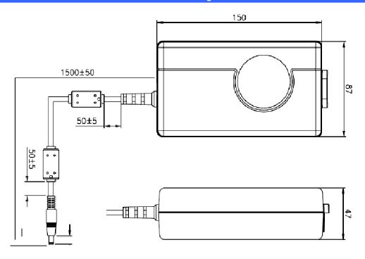
Dimensions are in mm. "#3" Connector shown.
