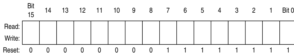
Figure 4-4. Stack Pointer (SP)
