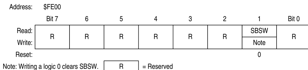
Figure 21-6. SIM Break Status Register (SBSR)
