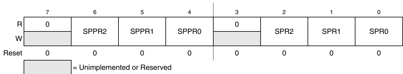
Figure 13-7. SPI Baud Rate Register (SPIBR)
