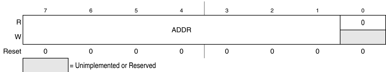
Figure 13-3. IIC Address Register (IIC1A)
