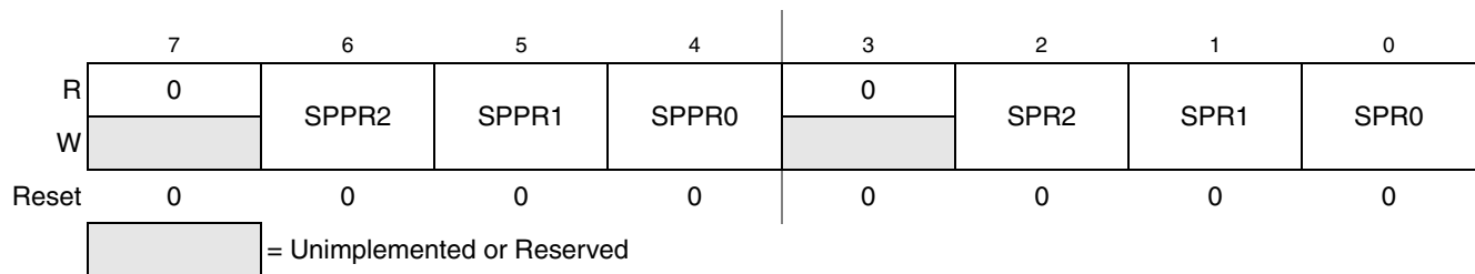
Figure 12-7. SPI Baud Rate Register (SPI1BR)
