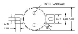
This transformer operates in the 20 Hz to 20 KHz range. The metal can provides excellent shielding from a broad range of external sources. While the nickel core provides high permeability combined with low losses.
