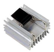
Ohmite's R2 Series (patent pending) heatsink provides a large surface area along with our C Series clipping mechanism to attach to a T0-220, T0-247, or T0-264 package. The self-aligning features of the clip assure secure attachment and enhanced thermal performance. Because no screws are required for device mounting, additional fins can be added to the rear side of the heatsink for increased total surface area in a more compact space.
