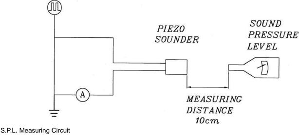
Input Signal: 10 Vp-p, 4.0 KHz, square wave Mic: RION S.P.L. meter UC30 or equivalent S.G.: Hewlett Packard 33120A function generator or equivalent
