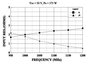
SERIES LOAD IMPEDANCE vs FREQUENCY
