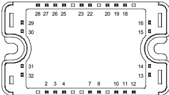
All multiple inputs and outputs must be shorted together
