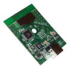
for most applications.) The SIPP firmware in the DLP-RF1 resides at the application layer and is based on Freescale's SMAC. The SIPP firmware provides basic access to DLP-RF1 functionality: packet receive and transmit, transceiver settings, EEPROM access, etc.
