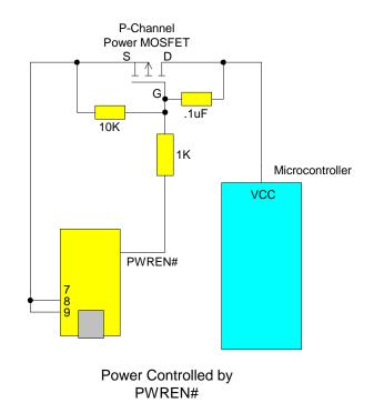
Figure 4 shows how to use a discrete P-Channel MOSFET to control the power to external logic circuits. This "soft-start" circuit accommodates designs that draw more than 100mA at power up.
