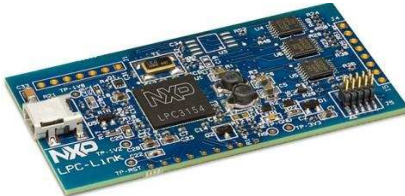
Figure 3-7 LPC-Link debugger module
