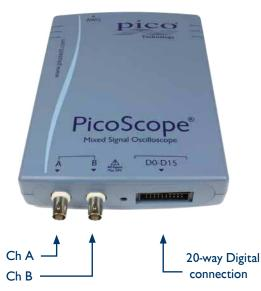
The front panel of the PicoScope 2205 MSO has two BNC analog input channels and a 20-way connection for up to 16 digital signals.
