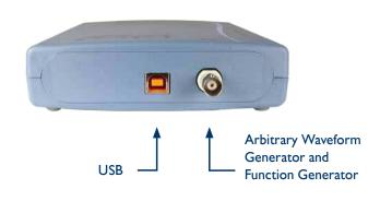
The rear panel of the PicoScope 2205 MSO has two connections: a USB port for connection to the PC, and a BNC for the AWG/Function Generator connection.
