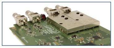
Careful front-end design and shielding reduces noise, crosstalk and harmonic distortion. Years of oscilloscope experience leads to improved pulse response and bandwidth flatness.
