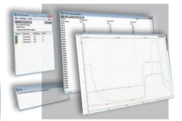
In addition to the monitor view, PicoLog can also display a graph, a spreadsheet and user notes. It can display them all at once, as shown here, or individually in any combination.
