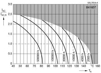
Useful life depending on case temperature  $T_{\text{C}}$  under ripple current operating conditions at  $V_{\text{R}}{}^{1)}$
