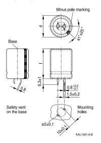
Snap-in terminals, length (6.3 ±1) mm. Also available in a shorter version with a length of (4.5 1) mm. PET insulation is marked with label "PET" on the sleeve.
