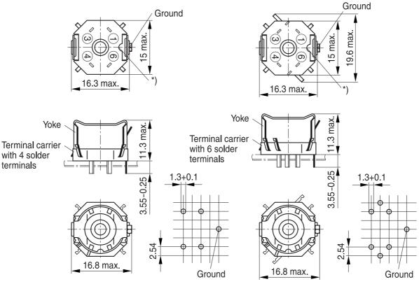
\*) This recess must be on the side of the grounding pin to ensure that the yoke locks in position.
