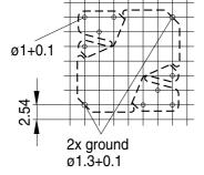
Hole arrangement View in mounting direction
