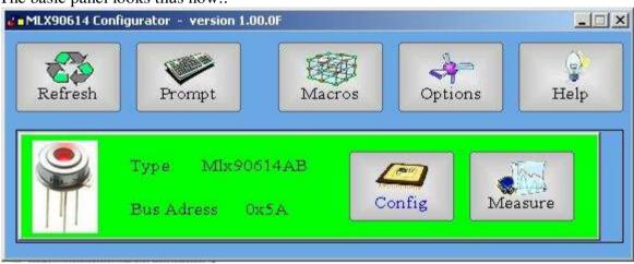
When USBEVB is attached to a usb port a LED on pcb board shines **BLUE**. When start program the SW **automatically** recognizes the module type(single or dual zone) ,SMBus address and power supply(3 or 5 Volts) and turns on it and the LED shines **GREEN**.
