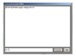
The button **Promt** opens a window from which you can manually send commands to USBEVB. The commands supported by USBEVB you can find in attachments (PromtComands.xls).
