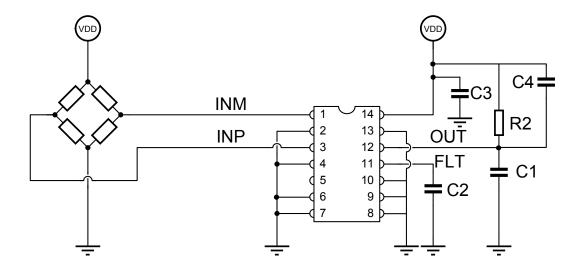
C1, C2, C3, C4 and R2 have the same values as for the ratio-metric application with use of external temperature sensor.
