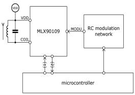
(1): MODE/SPEED config settings (2): DATA/CLOCK outputs
