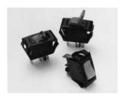
The LR-Series Curvette single pole illuminated miniature snap-in rocker switches are available with a rocker or paddle actuator. These lighted switches are available in a number of lamp voltages with internationally approved current ratings up to 16 amps. Due to the patented mounting ear design, these switches are compatible with a wide range of standard panel cutouts.
