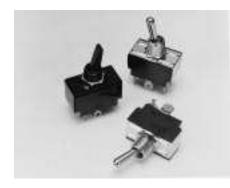
The G-Series toggle switches are single or double pole, AC rated up to 20 amps and contain a slow-make, slow-break contact mechanism. These switches are available in a wide range of ratings, terminations, circuits and bushing/toggle configurations.
