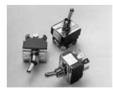
The H-Series toggle switches are heavyduty, high voltage, high amperage, threepole switches. These switches have a slow-make, slow-break contact mechanism, are AC rated to 600V, and are available in a wide range of ratings, circuits, terminations and bushing/toggle configurations.
