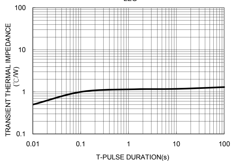
FIG. 6 TYPICAL TRANSIENT THERMAL IMPEDANCE PER LEG
